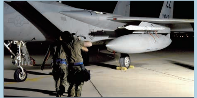
Airmen from the 378th Expeditionary Operations Group conduct an integrated combat turn to test their capability to land, refuel, weapons reload and take off at Prince Sultan Air Base, Kingdom of Saudi Arabia, July 3. An integrated combat turn allows the fighter jet to land, refuel and weapons reload in a rapid rate. This process allows for the fighter jet to spend less time on the ground and more time in combat operations directly supporting agile combat employment.
