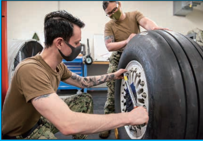
(U.S. Navy photos by Mass Communications Specialist 2nd Class Matthew Dickinson) ^ Aviation Structural Mechanic Airman Julian Denerson, from Clemmons, N.C., assigned to Aircraft Intermediate Maintenance Department (AIMD) Detachment Kadena, checks the torque on the nuts of a main landing gear tire from a P-8A Poseidon aircraft, April 21.
