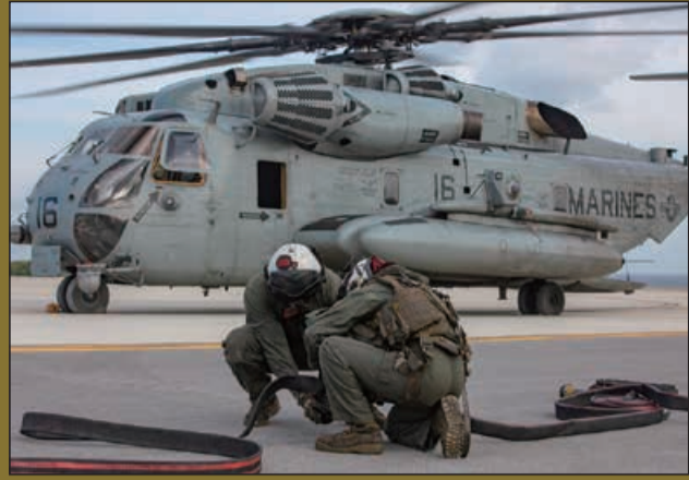
◀ U.S. Marines with Heavy Helicopter Squadron 466 set up fuel hoses as part of a forward arming and refueling point at le Shima Island, Jan. 7. A FARP is a temporary set up that rapidly arms and refuels aircrafts, allowing them to expedite the refueling process and to better operate in combat environments.
