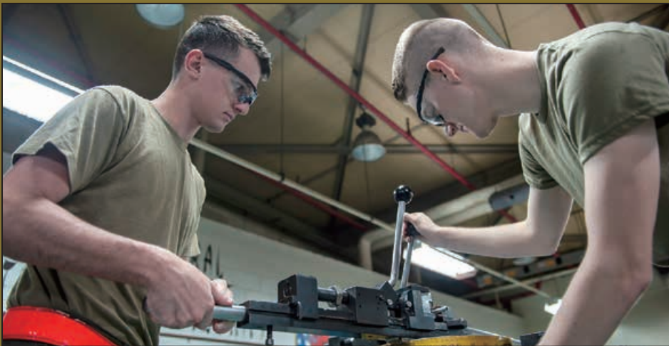
(U.S. Air Force photos by Naoto Anazawa) Airmen 1st Class Brady Motes (left) and Kyle Kirts (right), assigned to the 18th Equipment Maintenance Squadron aircraft structural maintenance journeymen, operate a production tube bender at Kadena Air Base, Oct. 4. As aircraft parts bend, break or corrode over time, the Airmen from the Aircraft Structural Maintenance flight step in to repair or replace the faulty equipment.
