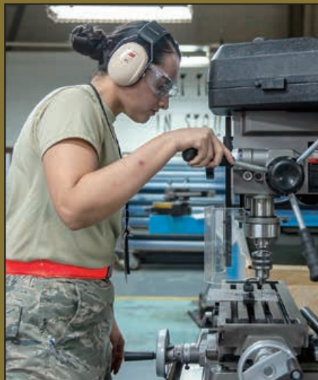
Airman 1st Class Amanda Pacheco, 18th Equipment Maintenance Squadron aircraft structural maintenance apprentice, drills holes into a metal plate.
