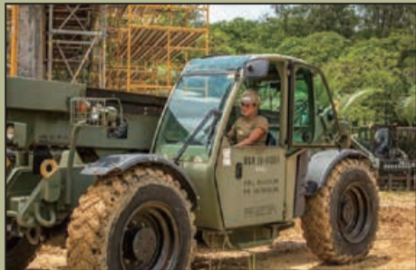
Equipment Operator Constructionman Sarah Ketchum, assigned to NMCB 4, prepares to lift assembled concrete formwork to the roof of the Explosive Ordnance Disposal storage building, Aug. 20.
