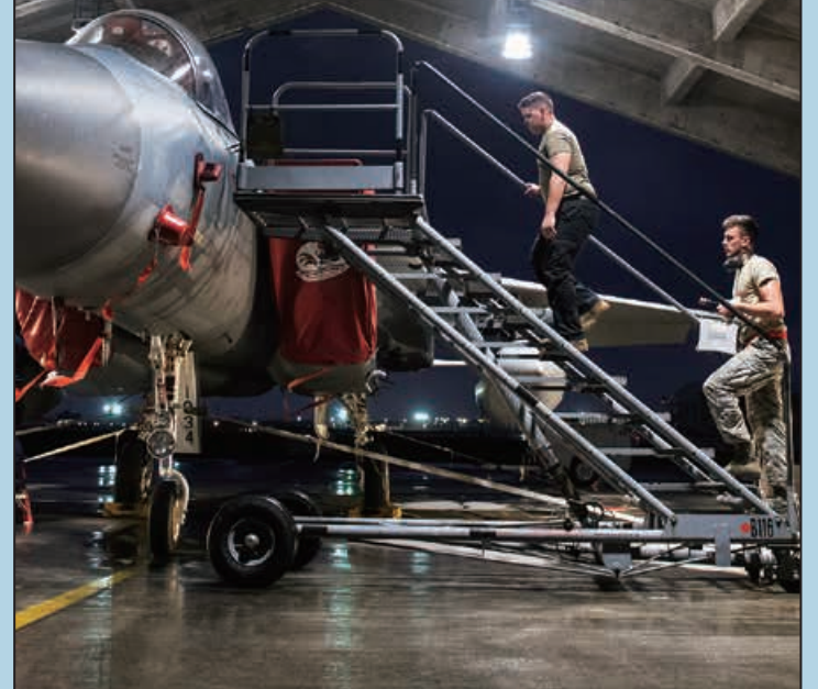
(U.S. Air Force photo by Tech. Sgt. Matthew B. Fredericks) U.S. Air Force Tech. Sgt. Michael Solomon, 18th Component Maintenance Squadron F-15 craftsman, left, and Airman 1st Class Grant McFall, 18th CMS F-15 apprentice, prepare to perform a 30-day egress final on an F-15C Eagle at Kadena Air Base, Sept. 19. During the routine inspection, the technicians check every component of the egress system for wear or damage, and any expired time-changeable parts are swapped out.
