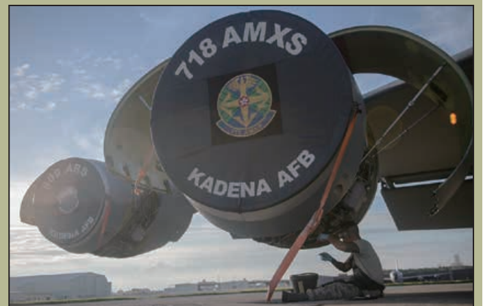
Senior Airman Derek Chau, 718th Aircraft Maintenance Squadron aerospace propulsion journeyman, prepares to drain fuel from the engine of a KC-135 Stratotanker during a routine inspection at Kadena Air Base, Sept. 26.
