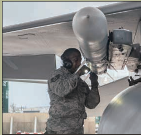
▲ A U.S. Air Force weapons load crew team from the 44th Aircraft Maintenance Unit attach an AIM-120 advanced medium-range air-to-air missile onto an F-15 Eagle during a quarterly weapons load competition at Kadena Air Base, July 1.
