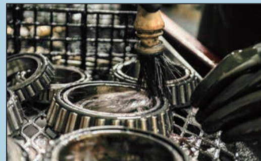
Senior Airman Landon Berry, wheel and tire technician assigned to the 18th Equipment Maintenance Squadron, presses a bearing cup into the nose wheel at Kadena Air Base, May 22. Aircraft tires must be periodically replaced so the wheel and tire shop takes those wheels, inspects and washes them so they can be reused.
