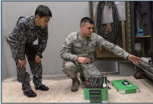
➤ Senior Airman Diana Garcia-Ferrufino, nondestructive inspection journeyman assigned to the 18th Equipment Maintenance Squadron, performs a metals check using the joint oil analysis program during a bilateral training exercise with the JASDF.
