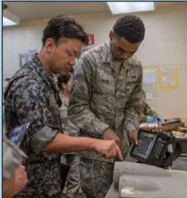
▲ Airman 1st Class Zacharius Shaw, nondestructive inspection apprentice assigned to the 18th Equipment Maintenance Squadron, demonstrates how to use an eddy current nortec 600 inspection unit during a bilateral training exercise with the JASDF May 23.
