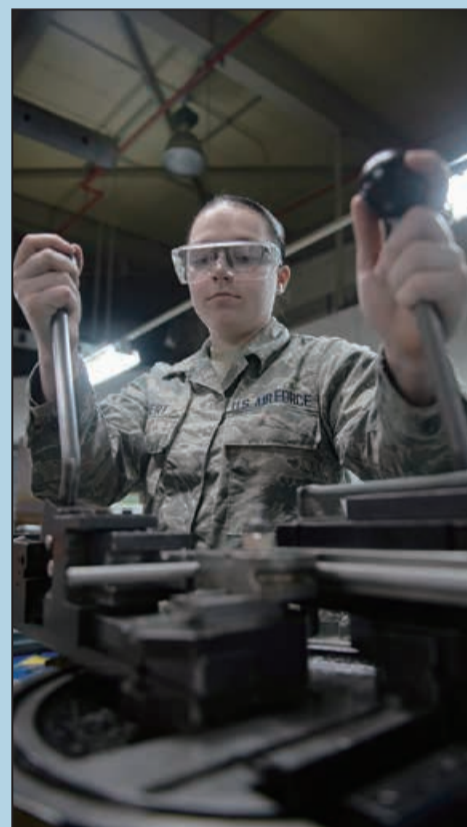
U.S. Air Force Airman Kristin Reichert, 18th Equipment Maintenance Squadron aircraft structural maintenance apprentice, bends metal tubing May 1, on Kadena Air Base. Aircraft structural maintenance Airmen train to understand the differences between metals and how they react to different types of stress.
