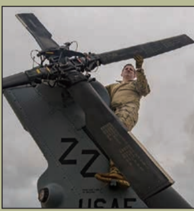
^ (Top photo) Senior Airman Chandler Hoskinson, 33rd Rescue Squadron special mission aviator, performs headspace and timing checks on the gun aircraft unit on an HH-60G Pave Hawk during pre-flight inspections May 8, on Kadena Air Base. (Bottom photo) Maj. Margaret McCord, 33rd Rescue Squadron flight lead, performs avionics system checks on an HH-60G Pave Hawk May 8.
