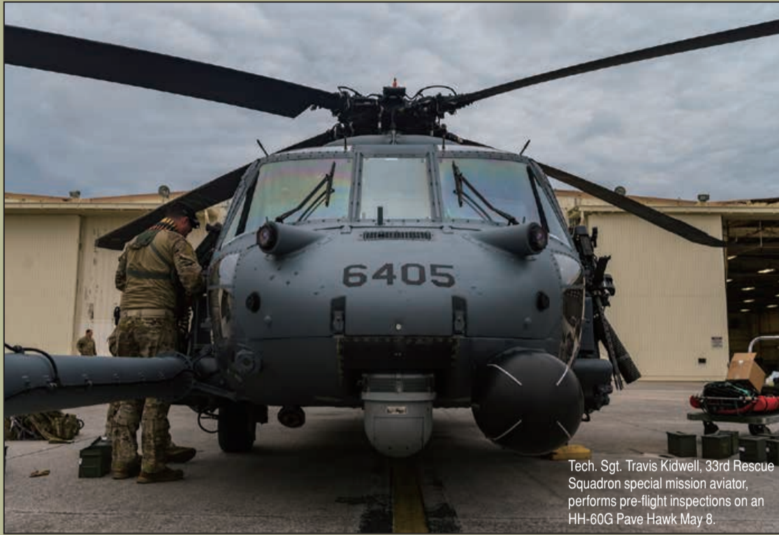
Tech. Sgt. Christopher Kersey, 33rd Rescue Squadron instructor special mission aviator, inspects the tail rotor paddles on an HH-60G Pave Hawk during pre-flight inspections May 8, on Kadena Air Base. The 33 RQS's primary mission lies in combat search and rescue as well as medical evacuation in a wartime environment.
