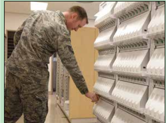
Tech. Sgt. Ryan Marr, 18th Medical Group pharmacy NCOIC, fills a prescription bottle from a pill-counting machine Sept. 10, at Kadena Air Base. Technicians use automated machines to count prescriptions involving large quantities of tablets to expedite their processes.
