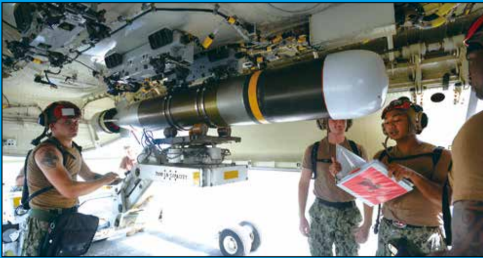
Aviation Ordnancemen assigned to the "Skinny Dragons" of Patrol Squadron (VP) 4 load a Mark 54 torpedo on a P-8A Poseidon aircraft during a proficiency exercise on Kadena Air Base, June 28.
