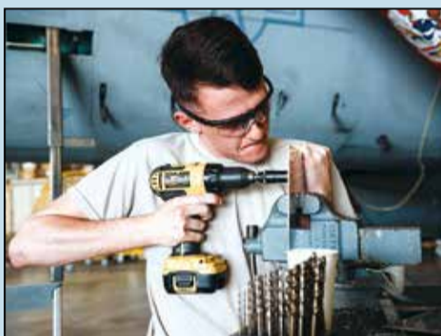
Airman 1st Class Brady Motes, 18th Equipment Maintenance Squadron aircraft structural maintenance technician, drills holes into a metal plate April 5, at Kadena Air Base. The 18th Equipment Maintenance Squadron helps maintain the two F-15 Eagle squadrons stationed at Kadena.
