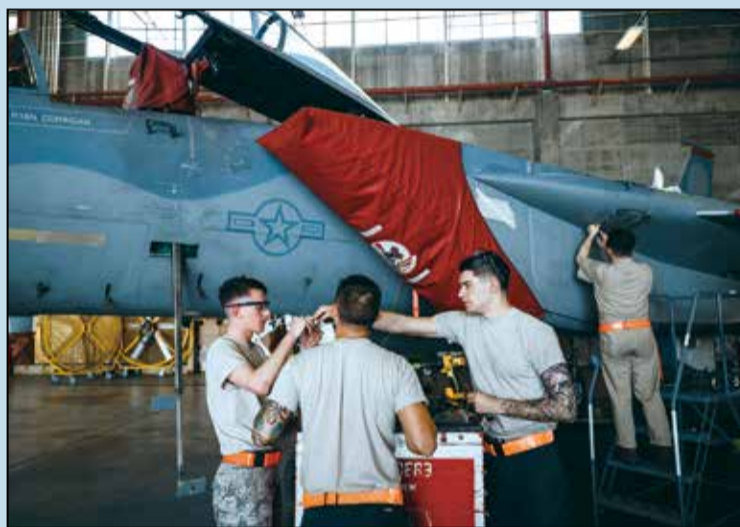
Airmen from the 18th Equipment Maintenance Squadron install a patch onto an F-15 Eagle April 18, at Kadena Air Base. The 18th EMS ensures Kadena's aircraft are structurally sound to fly.
