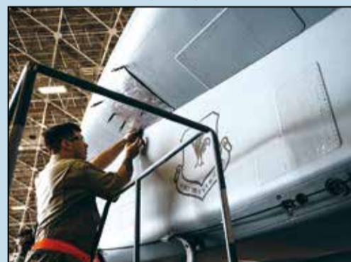
Senior Airman Michael Bock, 18th Equipment Maintenance Squadron aircraft structural maintenance technician, fastens a metal plate to an F-15 Eagle April 5, at Kadena Air Base. Structural maintenance technicians work directly from their technical orders to create, repair or maintain required aircraft parts.
