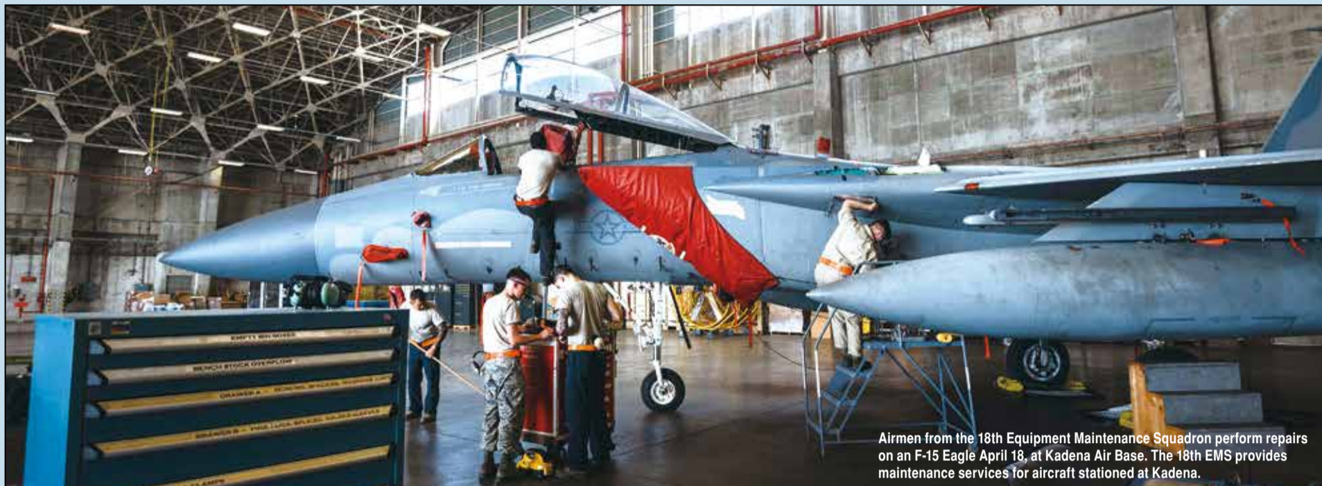
Airmen from the 18th Equipment Maintenance Squadron install a patch onto an F-15 Eagle April 18, at Kadena Air Base. The 18th EMS ensures Kadena's aircraft are structurally sound to fly.
