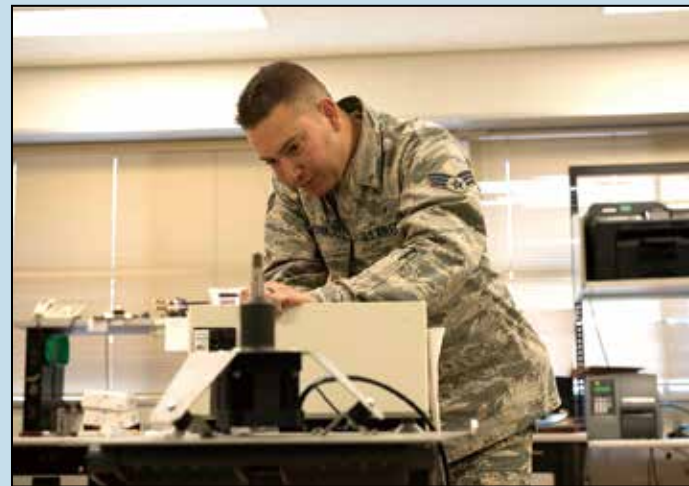
Senior Airman Randy Maldonado, 18th Medical Group biomedical equipment technician, repairs a centrifuge March 21, at Kadena Air Base. A centrifuge is used to separate the different components within a blood sample. This allows technicians to test the appropriate areas for more intricate procedures.
