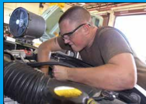
(U.S. Navy photo by Construction Mechanic 2nd Class Jeremy Colbert) Construction Mechanic Constructionman Gabriel McGraw assigned to NMCB 4, replaces the idler pulley on a Light Service Support Vehicle, Jan. 18, at Camp Covington, Guam.
