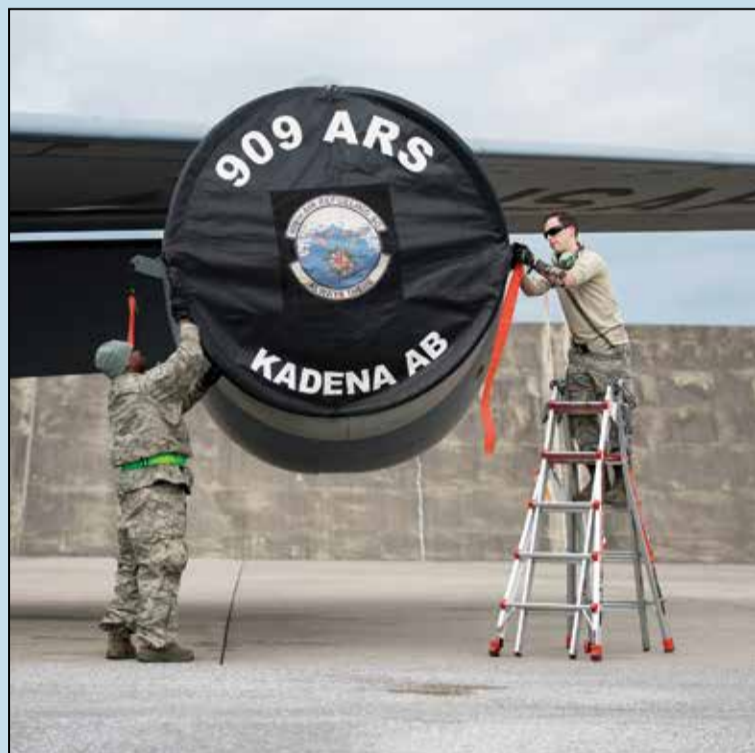
^ Tech. Sgt. Bill Smith (left) and Senior Airman Christoffer Horner, 909th Aircraft Maintenance Unit KC-135R crew chiefs, place engine covers onto a KC-135R Stratotanker.
