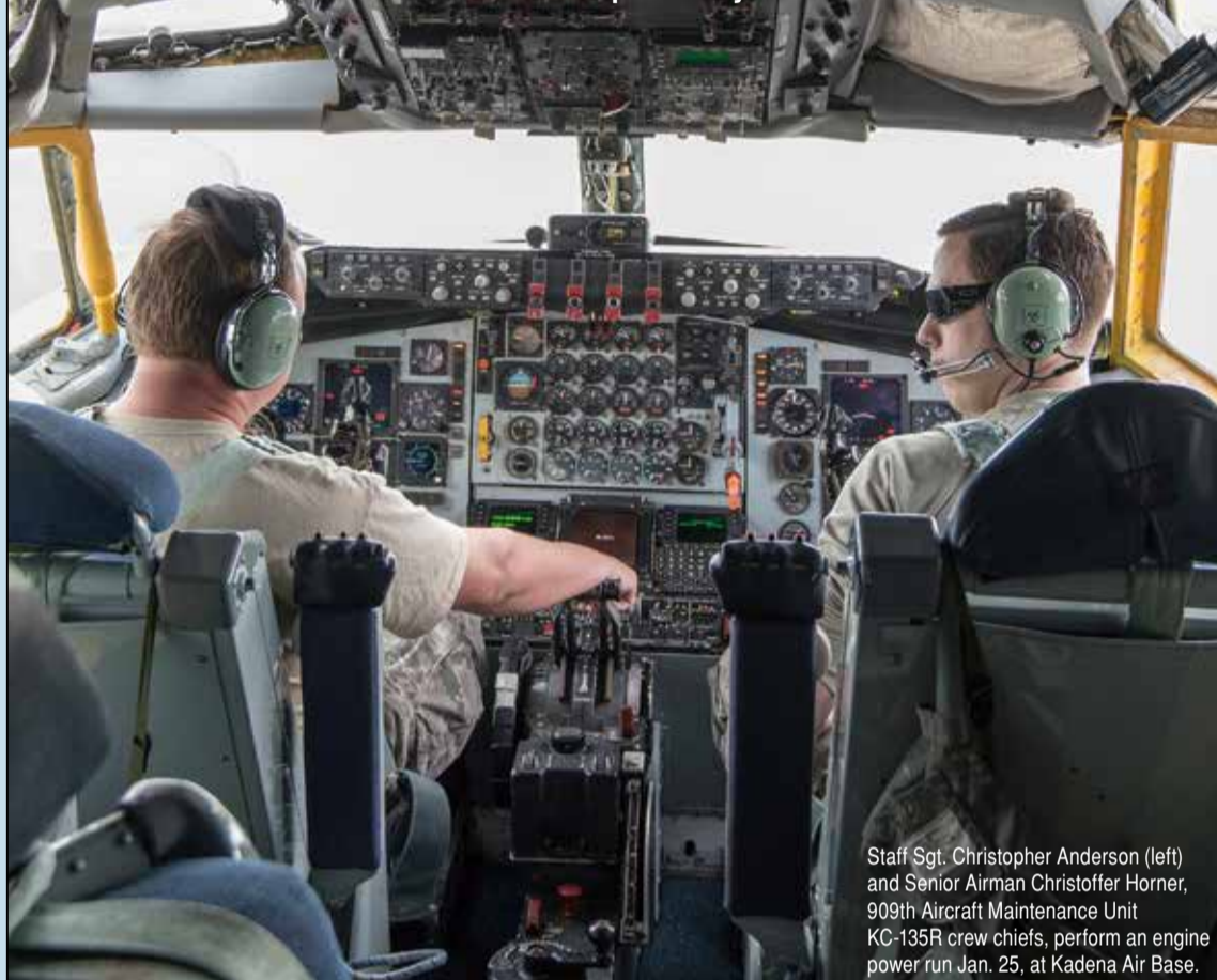
^ KC-135R crew chiefs from the 909th Aircraft Maintenance Unit, perform an engine power run Jan. 25, at Kadena Air Base. KC-135R Stratotanker crew chiefs look for discrepancies such as leaks, smoke or damage during a power-run.
