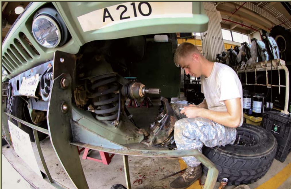
A wheeled vehicle mechanic Soldier with 1st Battalion, 1st Air Defense Artillery Regiment, makes repairs to a High Mobility Multipurpose Wheeled Vehicle (HMMWV) tire hub on Kadena Air Base, Oct. 18.
