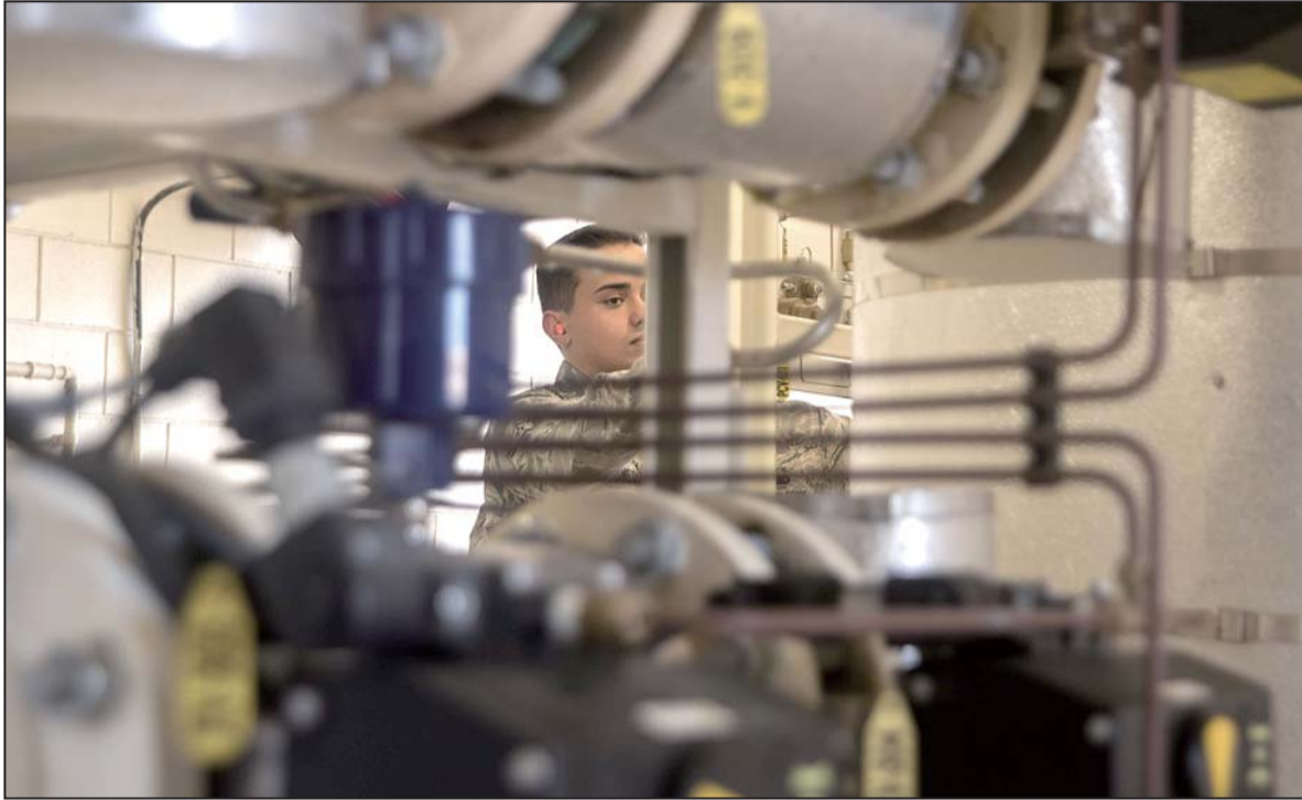
◀ Airman 1st Class Olavio Benito, 18th Logistics Readiness Squadron cryogenic production technician, recalibrates an oxygen purity analyzer Sept. 12, at Kadena Air Base. Oxygen is run through a machine removing all of the moisture from the air before being cooled to -300 degrees Fahrenheit. This cooling causes the gaseous oxygen to turn into a compact, liquid form used by pilots and medical personnel. Cryogenic production technicians require that all of the liquid oxygen produced in their facility have a minimum purity of 99.5 percent.
