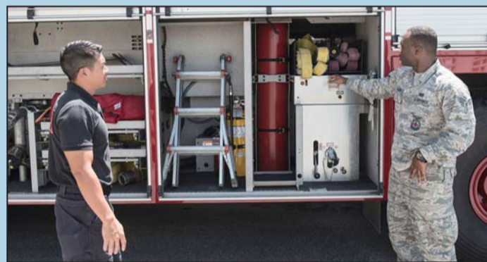
▲ Yuhei Tajima and Senior Airman Korey Wilson, 18th Civil Engineer Squadron firefighters, inspect the equipment bay of an Oshkosh Striker 6x6 July 20 at Kadena Air Base. The Oshkosh Striker 6x6 has a max speed of 72 miles per hour and can traverse the length of Kadena's runway in less than 2 minutes.
