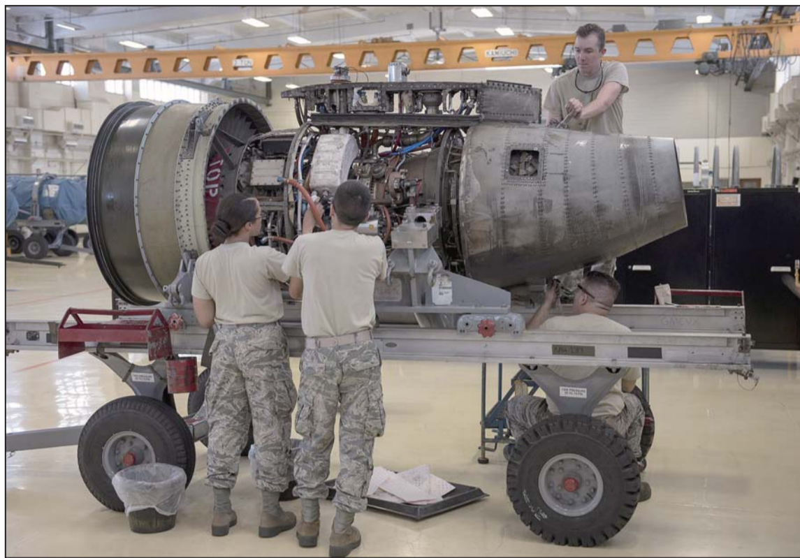
▲ Aerospace propulsion technicians from the 18th Component Maintenance Squadron service an A-10 Thunderbolt II engine July 6, at Kadena Air Base. The Airmen performed preventative maintenance, which requires them to completely deconstruct the engine prior to rebuilding it. (U.S. Air Force photo by Senior Airman John Linzmeier)
