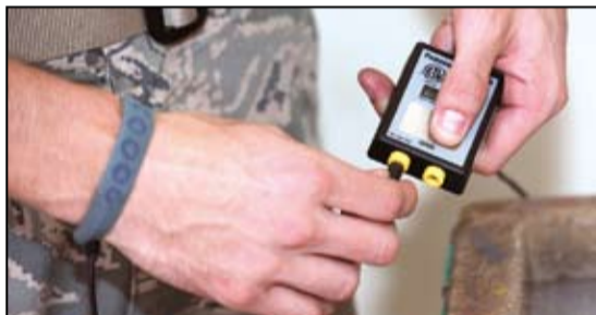
◀ Airman 1st Class Cody Lasagna, 18th Munitions Squadron crew member, grounds himself with an antistatic system on Kadena Air Base, Sept. 4. When working with active munitions, Airmen are required to periodically ground themselves to remove any buildup of static electricity that could potentially detonate the assets.
